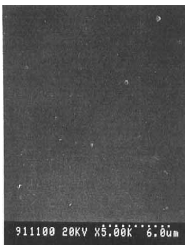
FIGURE 3 SEM image of polyimide LB film deposited on HOPG substrate
